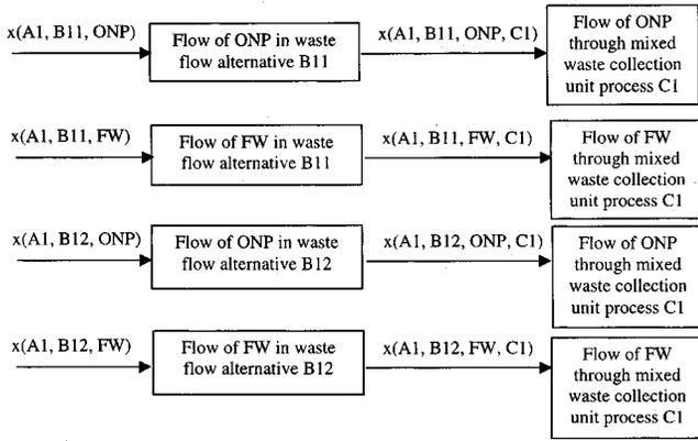
**Fig. 6.** Mass balances for individual waste items handled in collection combination A1
