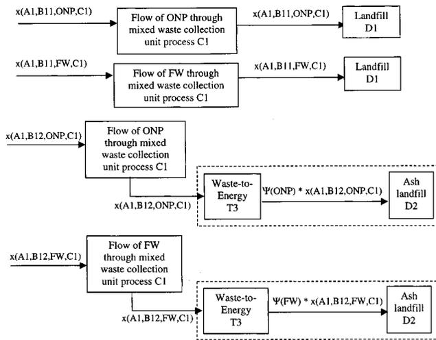
**Fig. 7.** Mass balances for waste handled by collection unit processes in collection combination A1
