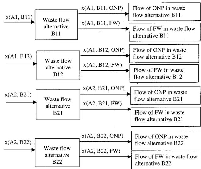
Fig. 5. Mass balances for waste flow alternatives
